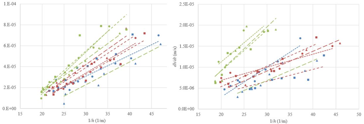
**Figure 2:** Example linear fits of Equation 1, for compressed glass weft (left) and carbon warp (right); blue = 41/50% fiber (glass/carbon), red = 45/55%, green = 51/60%
