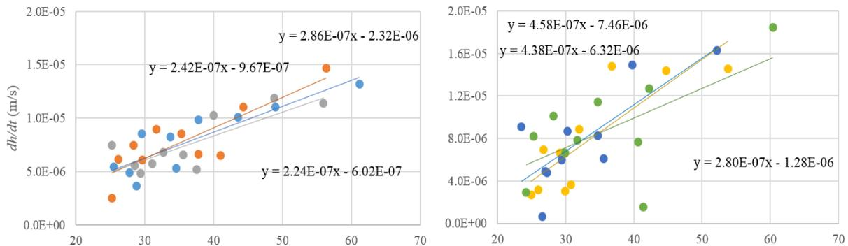
**Figure 1:** Example linear fits of Equation 1, for uncompressed carbon warp (left) and weft (right) flow directions.
